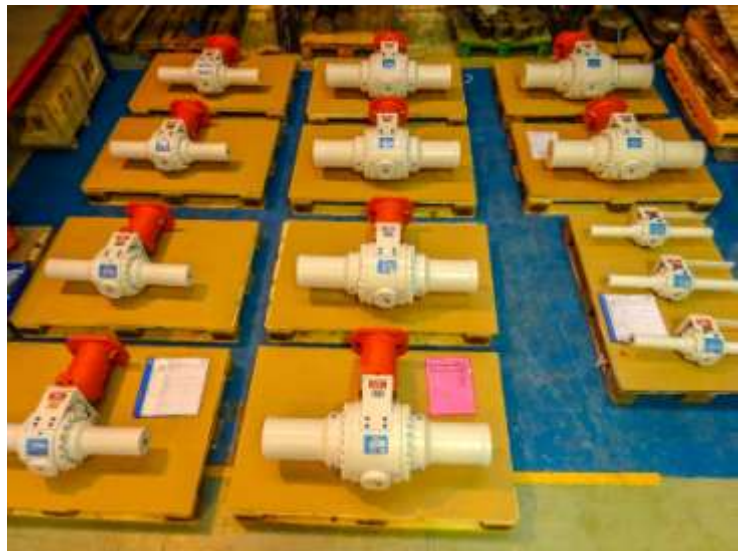
2”, 4” and 6” Ball Valves API 6D, 300#, 316SST Body c/w FF Trim, SCH 40 Butt Weld End Connections, ROV - BS EN 13628-8 FIG18.CL4
